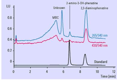
Figure 34 Qualitive analysis of MBC (2-benzimidazole carbamic acid methylester) and impurities
