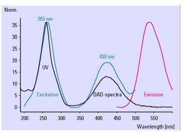
Figure 33 UV-spectrum and fluorescence spectra for 2,3-diaminophenazine (DAP)
