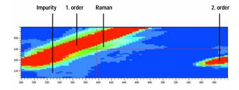
A pure water sample was put into the flow cell. Spectra were recorded at 5 nm step sizes.
