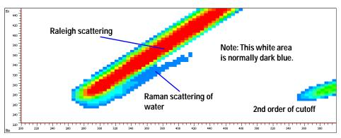
Figure 43 Fluorescence Scan of Water
