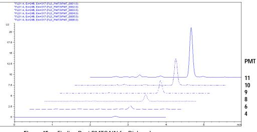
Figure 45 Finding Best PMTGAIN for Biphenyl
