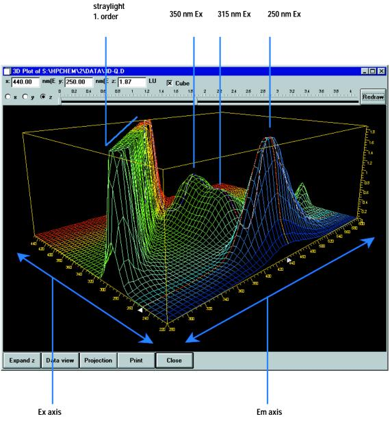
Figure 30 Characterization of a pure compound from a fluorescence scan
