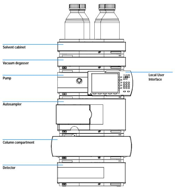
Figure 21 Recommended Stack Configuration (Front View)
