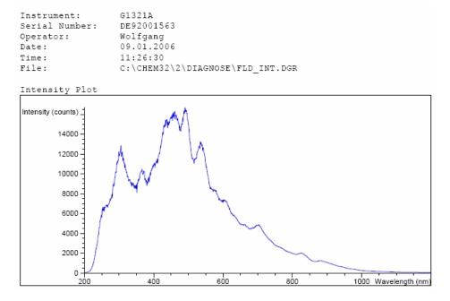
Figure 55 Lamp Intensity Test (Report)
