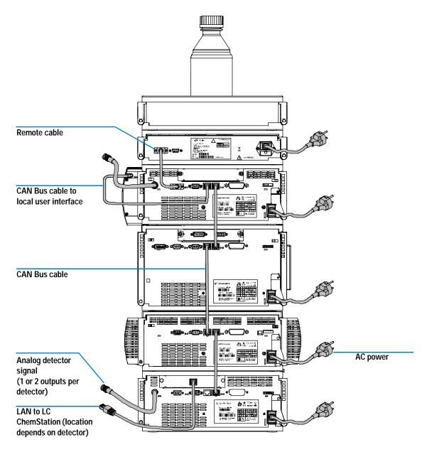
Figure 22 Recommended Stack Configuration (Rear View)
