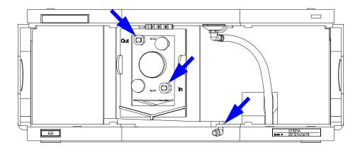
Figure 52 Observing for Leaks
