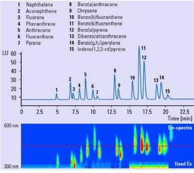
This shows the isofluorescence plot of emission spectra for 15 PNAs (5 µg/ml) with a fixed excitation wavelengths (260 nm).
