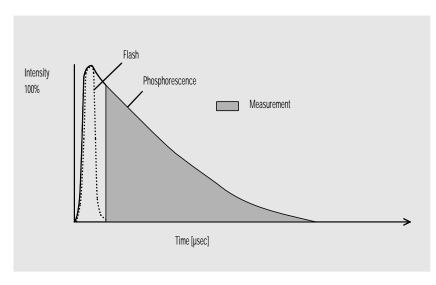
Figure 13 Measurement of Phosphorescence
