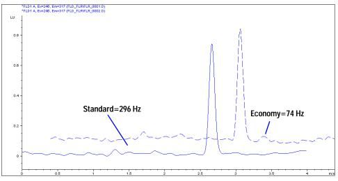
Figure 46 Xenon Flash Lamp Frequency
