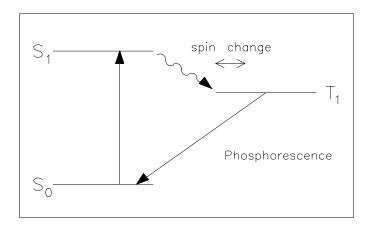
Figure 4 Phosphorescence Energy Transitions
