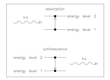
Figure 2 Absorption of Light Versus Emission of Light
