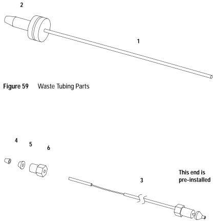
Figure 60 Inlet Capillary (Column-Detector) Parts
