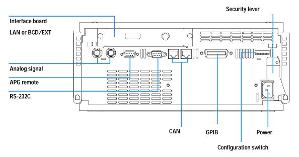
Figure 24 Rear View of Detector
