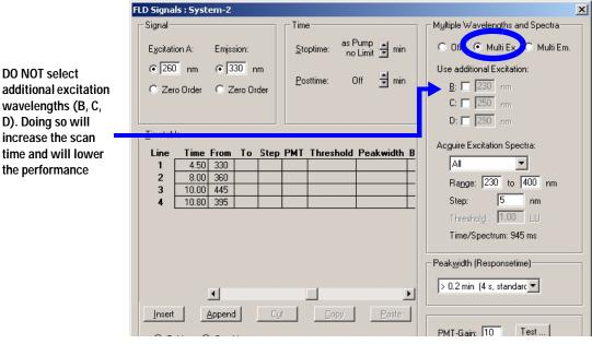
Figure 39 Detector Settings for Excitation Scan
